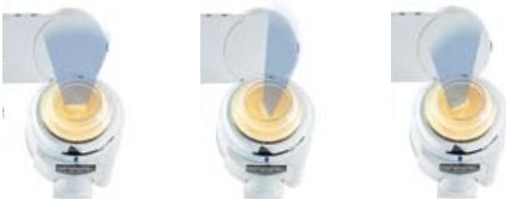
FarSight integrates a specially designed curved array transducer into the therapy head of the *Compact Sigma*. The integrated transducer allows for deep imaging while remaining outside the shockwave path at all times. The motorized transducer can be adjusted at the touch of a button to rotate along the longitudinal scanning plane.
